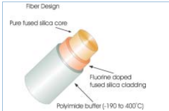
Figure 17 Fiber optic design
